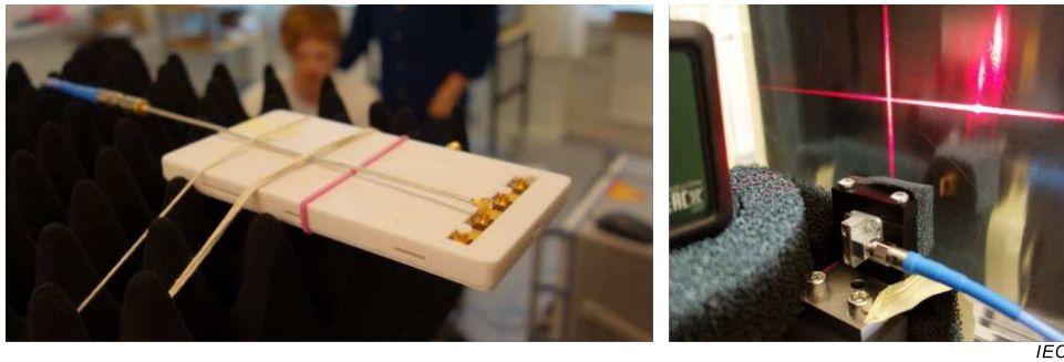
Figure H.13 – Mock-up with antenna port number 2 connected to the VNA (left) and the open waveguide probe and alignment system (right)
